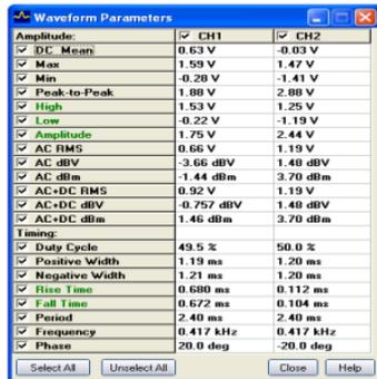
Open the waveform parameters window to see extended waveform parameters
