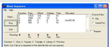
In "Tools" Open the Wave Sequence panel to create automated wave forms coming from file or serial port data scripts.
