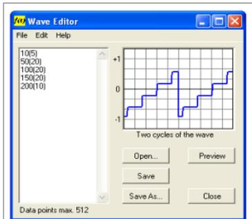
In "Tools" Open the Wave editor to generate your own waveform. In this example: level 10: 5 times, level 50: 20 times ...
